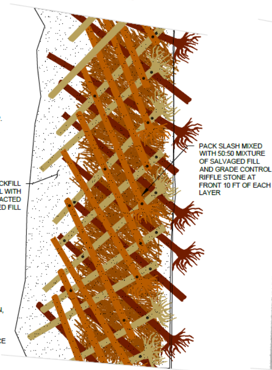
PLAN VIEW BACKFILL 3 & 4 LAYER CRIB WALL
